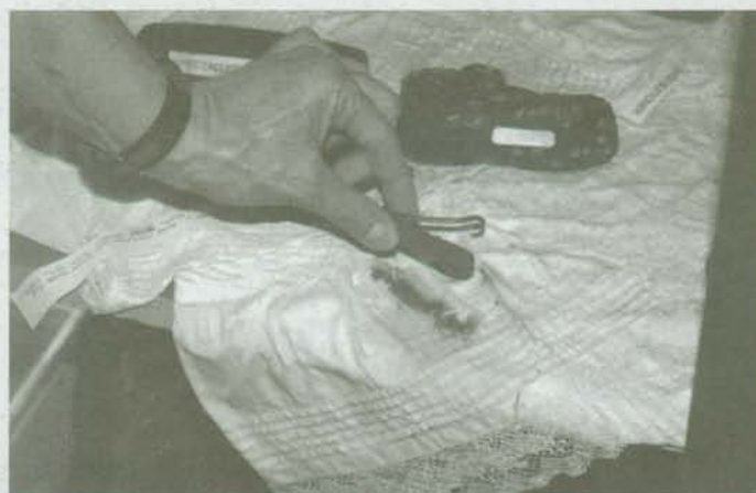
Rust developed on a damp textile after a metal artifact landed on it during Hurricane Katrina, Old Spanish Fort, Pascagoula, MS.
