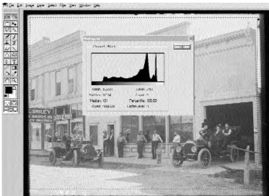
Histograms offer the best view of tonal range captured by the scanner and are examined for clipping as well as the correct setting of white and black points. Spiking on the ends of the histogram usually indicates clipping.
