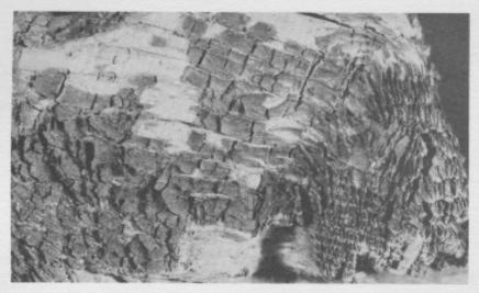
Advanced soft rot in oak framing from the whaler Charles W. Morgan. When dry, the wood appears charred, and small pieces flake off. (In other instances soft-rotted wood may appear only a "weathered" gray.) Microscope examination usually is required to confirm soft rot. Since this type of decay is a surface phenomenon, the wood retains much of its original strength.
