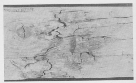
Advanced brown cubical rot in a pine board from the sub-flooring under a bath-tub. Note that as brownrotted wood dries, it shrinks and cracks across the grain into small cubes, much like charcoal. The wood usually will have a tan to brown coloration, noticeably darker than that of sound wood. Strength loss is almost total.
