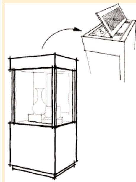
**Integral case lighting. Isolate case-mounted lighting fixtures and lamps in a separate lighting chamber. Dissipate heat from the lights with vents; electric fans may be required, especially in a large case. Use a heat-reflecting glass for the transparent layer between the lights and display chamber or use double-glazed construction.**
