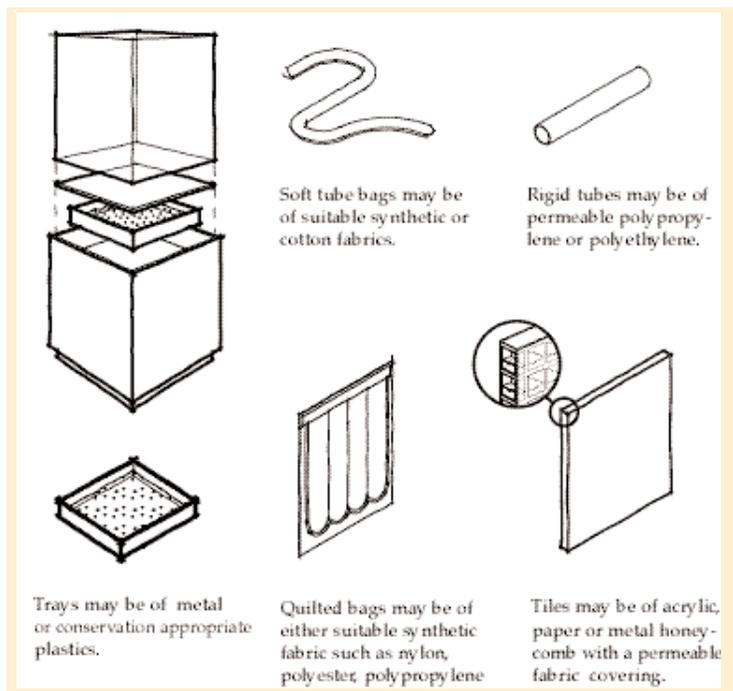
**Passive humidity control.** The maintenance chamber holds either loose silica gel contained in a tray or in mesh bags, silica-impregnated cassettes, tiles, paper, or foams. Generic silica gel desiccant is useful for maintaining relative humidity between 30 and 40%. Newer, hybrid silica gels are better for a middle range of 50 to 60% relative humidity.
