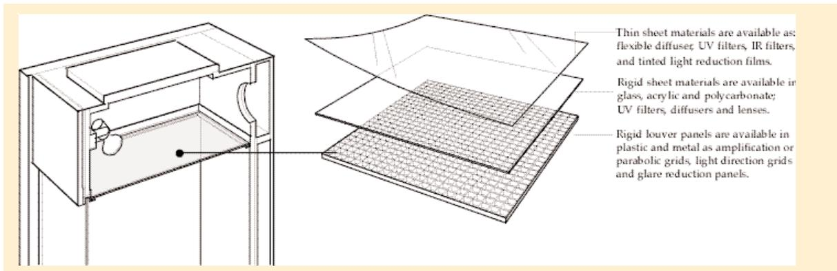
**Reduce the amount of light and heat passing through the glazing panel with filters and light-directing and -controlling devices. Using metal rather than wood to construct the lighting chamber will help dissipate heat.**
