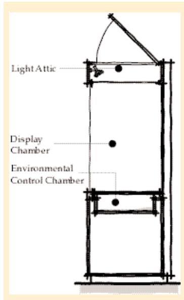
**Three chambers of a case: display, lighting, and maintenance or control. Isolate lighting fixtures from the display chamber with a transparent glass or acrylic panel sealed with a gasket or caulk. If a micro-climate will be maintained, locate silica gel or equipment in the maintenance chamber. Provide access panels or doors for staff to service the lighting and maintenance chambers.**
